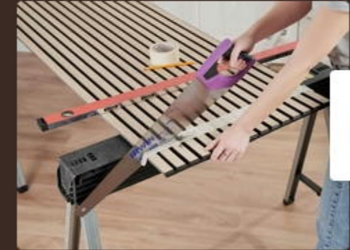
Step 3. Use a fine tooth saw to cut the panel along the marked line.
