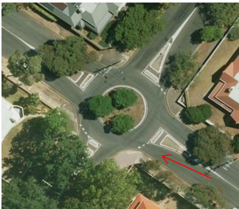
Photo 34: Tangential Roundabout at Winchester Street/ Fourth Avenue – faster speed (note: arrow shows direction of motor vehicle)
