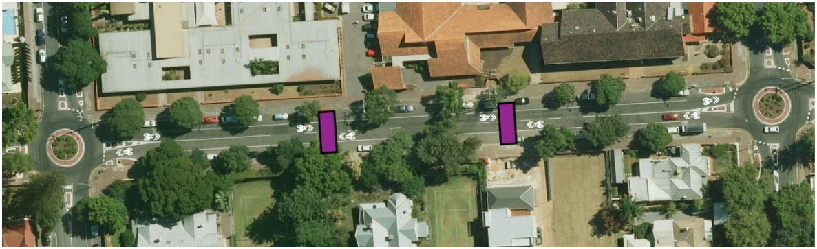
Figure 17: Illustration of Beulah Road with approximate location of traffic calming options and sharrows between roundabouts
